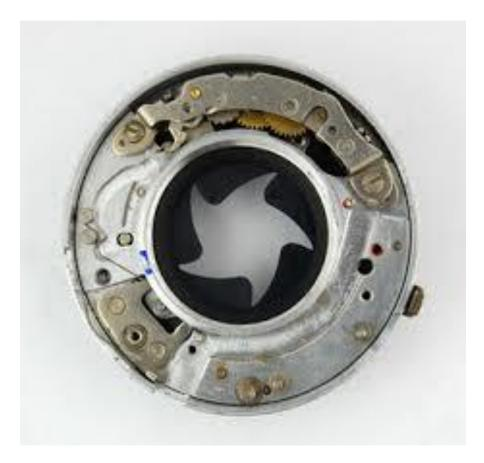
The leaves simultaneously snap open, stay open for the predetermined time (shutter speed) and then snap shut and if you are using flash it will fire when the shutter is completely open regardless of shutter speed.
